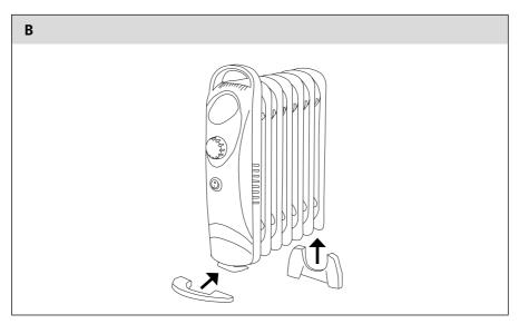
After attaching the feet A(6), check the stability of the heater on an even, dry and firm surface.
