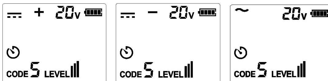
Figure 7.1.2b Voltage below 30V
