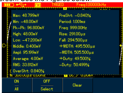
Figure 6-16A UTD1000CL measures all parameters
