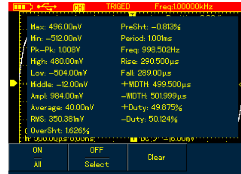
Figure 4-17A UTD1000CL measures all parameters
