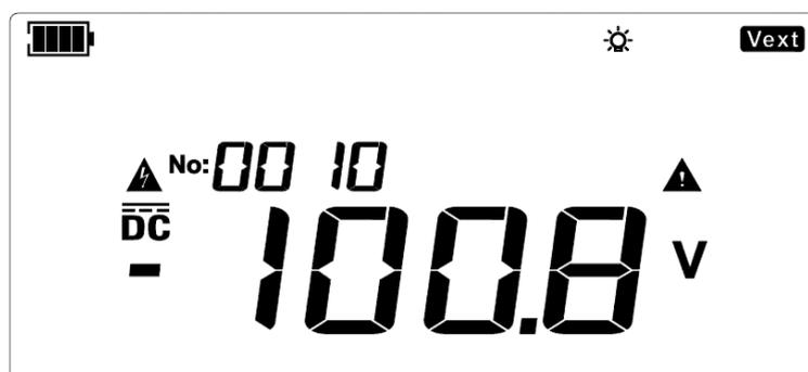
Figure 9.24 Negative DC voltage measurement
