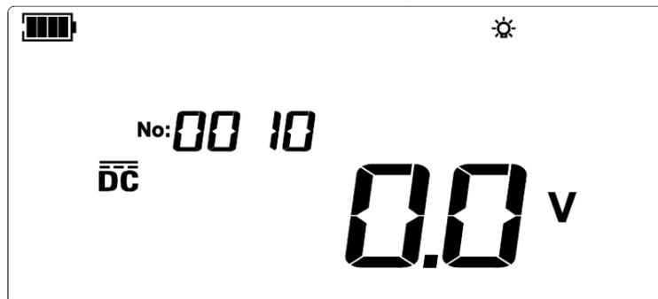
Figure 9.21 AC/DC voltage measurement (Default interface)
