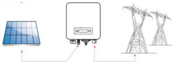
Figure2-1 PV Grid-tied System
