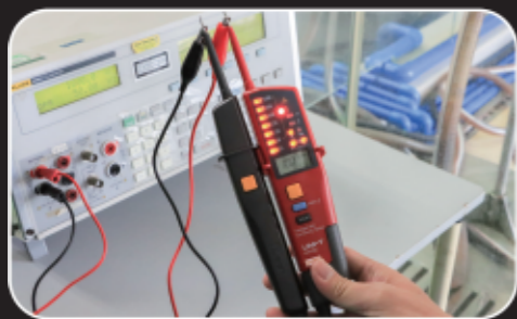
Voltage test: up to 1000V (AC/DC)
