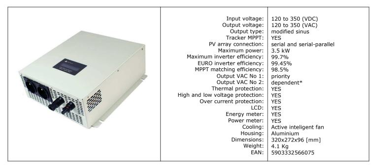
The ECO Solar Boost PRO MPPT-3000 inverter is designed to built heating system powered by solar energy as easy as possible. It is enough to connect PV array to input of the inverter and electric boiler to the output. By ECO Solar Boost PRO you can power any type of electric heater like electric boilers, heating mats etc.
