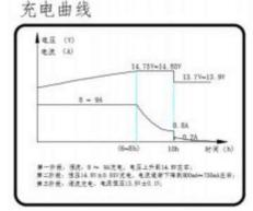
The standard temperature of this charging process is 20°C, as the temperature decreases or increases, the voltage adjustment coefficient is + or -0.018V/°C
